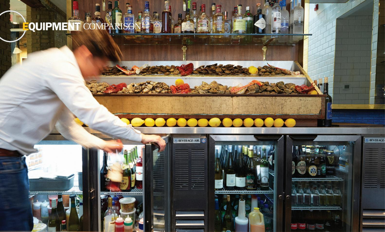
line with other under-bar equipment, coolers can be as shallow as 24-in.D but can go up to nearly 30-in.D.
