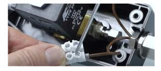
10. Carefully place the terminal block within the valve housing box. Close the cover using the four screws and tighten them securely.
