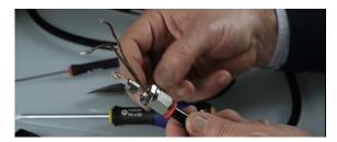
3. Temporarily disconnect the black tube from the connector by holding and pressing the red ring which will allow the tube to be released. Pull the tube until disconnected.
