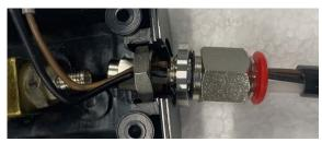
5. Tighten the end fitting with adjustable wrench until secure with the seated nut.
