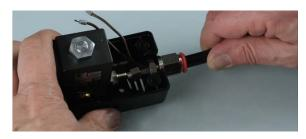
7. Attach the tubing male threads to the valve using the adjustable wrench. Do not over tightening the nut.
