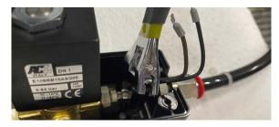
8. Insert the black and brown wires into the terminal block.
