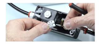
Use a flathead screwdriver to tighten the screws on the terminal block to secure the two wires.
