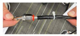
4. Loosen and insert the hex nut into its seat ensuring that the end fitting and spacer are outside of the valve housing.
