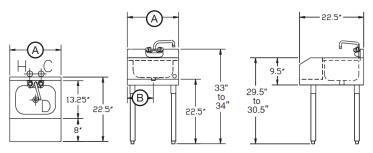
Mechanical Requirements: 1/2" IPS hot and cold water. 1-1/2" IPS drain connection.
