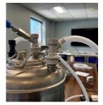
3. From the "Y" fitting, one line will go to the faucet, and the other will go to inlet on the pump. The tubing with the grey connection piece will connect to the outlet of the pump, and the connection piece will connect to the lid.
