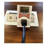
An outlet is required for the timer to plug into (preferably outside the direct draw box). The pump will plug into the timer, so you will need to drill a hole in the side/back of the box to fit the cord kit through.
