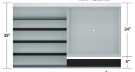
Adding a single speed rail to a KR24 unit will increase the depth 5" to match a KR29 unit.
