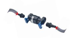
Install Inline Pressure Regulator to incoming water line. Two 3/8" hose barbs (included) snap into regulator. Plumb regulator to braided, high pressure, flexible tubing on both ends, and secure with Stepless stainless-steel clamp.
