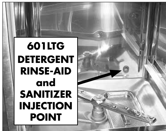
On the 601LTG, chemicals enter the wash tank through a fitting on the rear wall of the tank.
