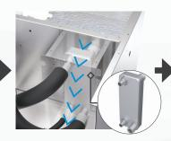
Glycol flows through the flat-plate to be rapidly cooled to optimal temperature before entering pumps.
